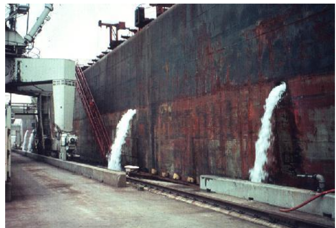
Fig. 1. Water ballast out in the port
