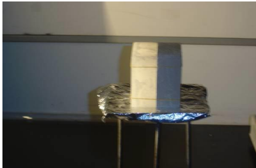
Fig.5. The photometer with aluminum foil between two pieces of paraffin. What the two paraffin pieces will look like if they receive different amounts of light.
