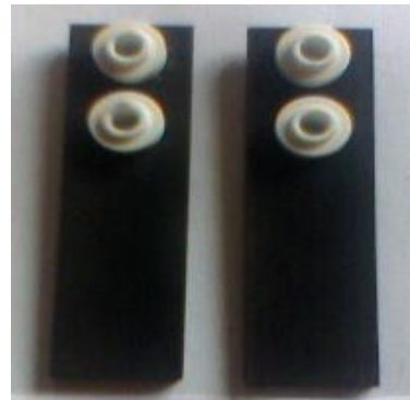
Fig. 11. CMP 07; gas medium; Dark sooty film with slight brownish superimposition, Corr. Rate, 0.4110 mpy, 0.3769mpy; View immediately after extraction.
