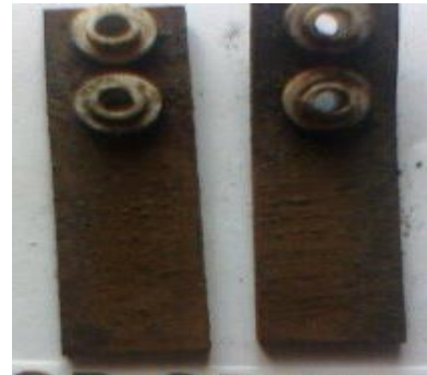
Fig.9. CMP 05; coupons immersed in recirculation water line. View immediately after extraction, campaign 1, dark brownish scales and water covering; average corr. rate, 2.7472 mpy
