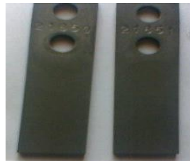
Fig. 10. CMP 09; gas medium; Smooth, waxy, ash coupons' surfaces, Corr. rate, 0.2033 mpy. View immediately after extraction.
