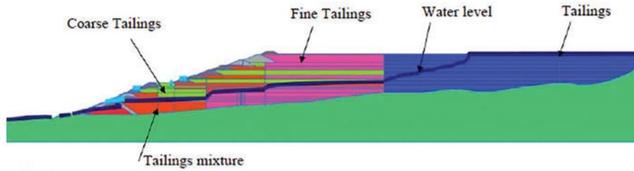
Fig. 12. Distribution of tailings in the cross-section [6].
