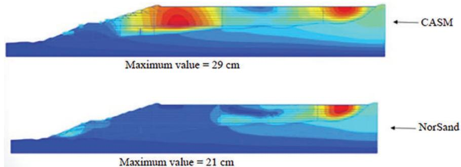
Fig. 14. Total displacements comparison between CASM and NorSand models
