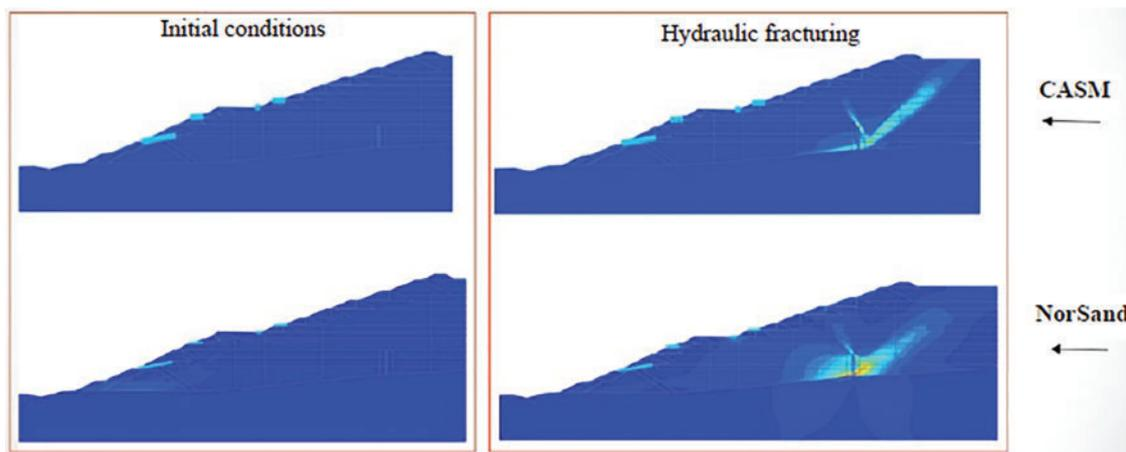
Fig. 19. Resulting shear strains in both CASM and NorSand models due to hydraulic fracturing.
