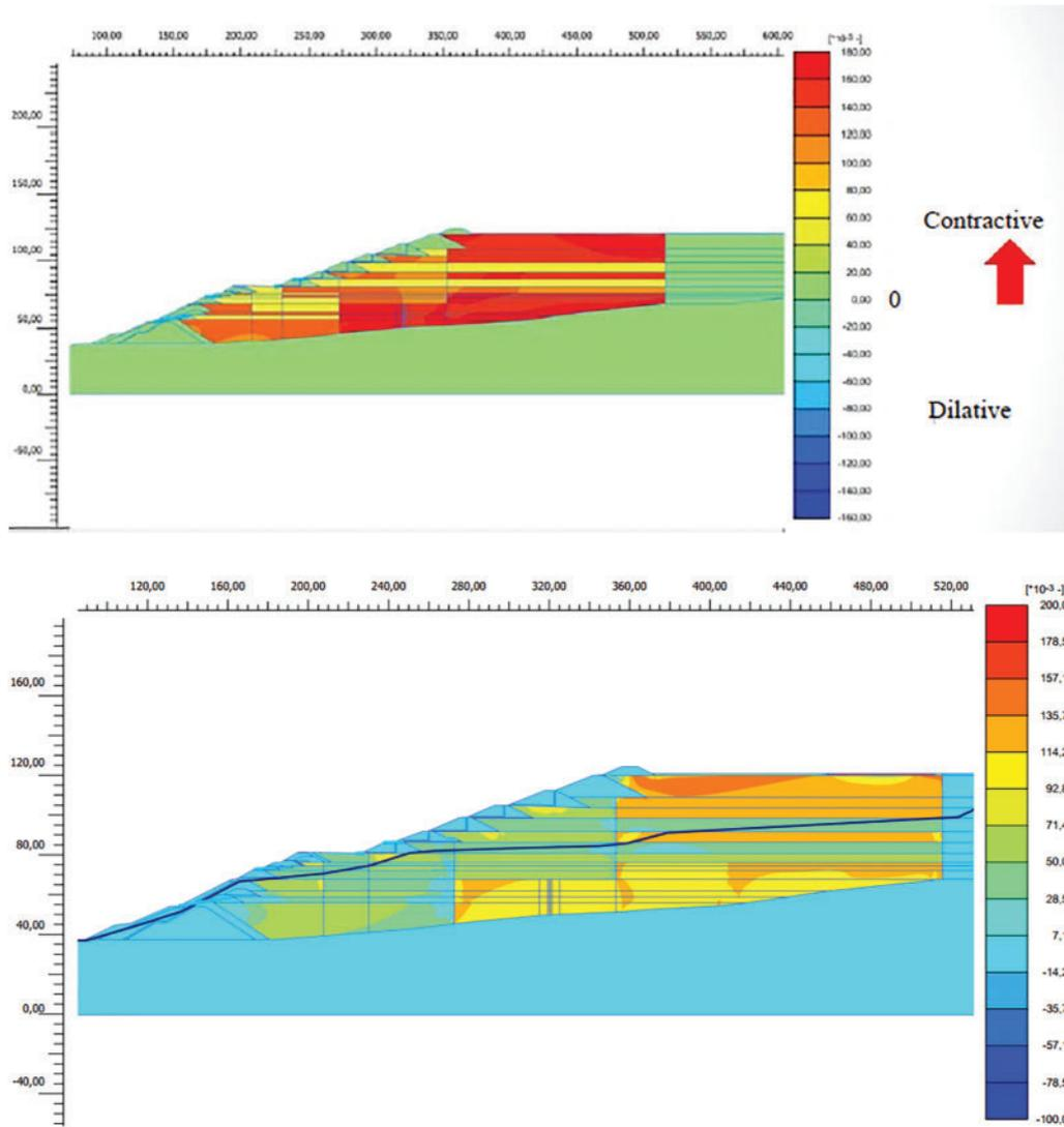
Fig. 16. State parameter, NorSand model (top) and CASM (bottom).
