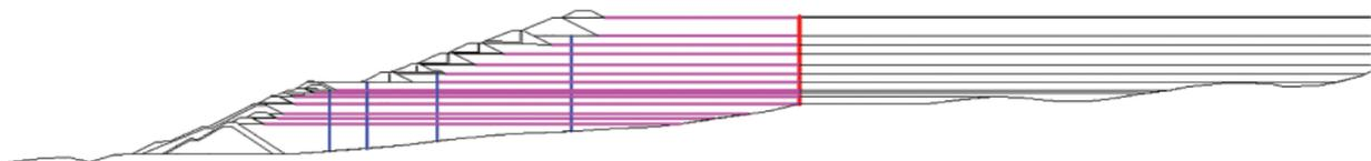
Fig. 10. Brumadinho Dam analysis cross-section.
