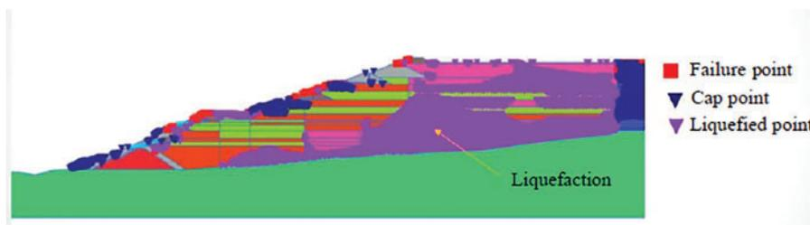
Fig. 17. Plastic points, NorSand model.
