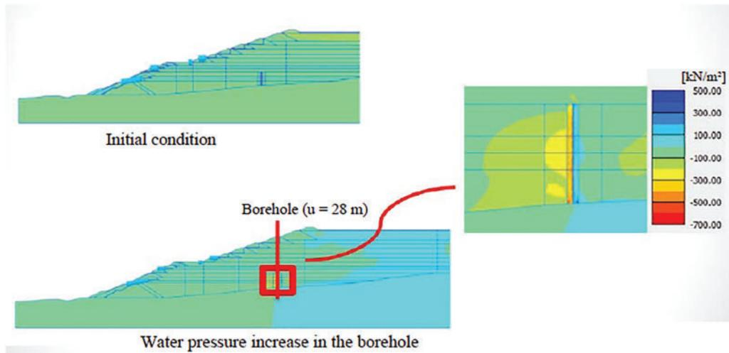
Fig. 18. Simulation of water pressure increase of 28 m head in the borehole.
