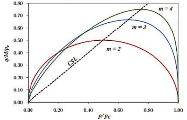
Fig. 6. Normalised plastic potential function for different  $m$  values [7].
