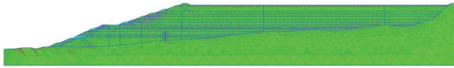
Fig. 13. Finite element mesh for Plaxis 2D analysis.
