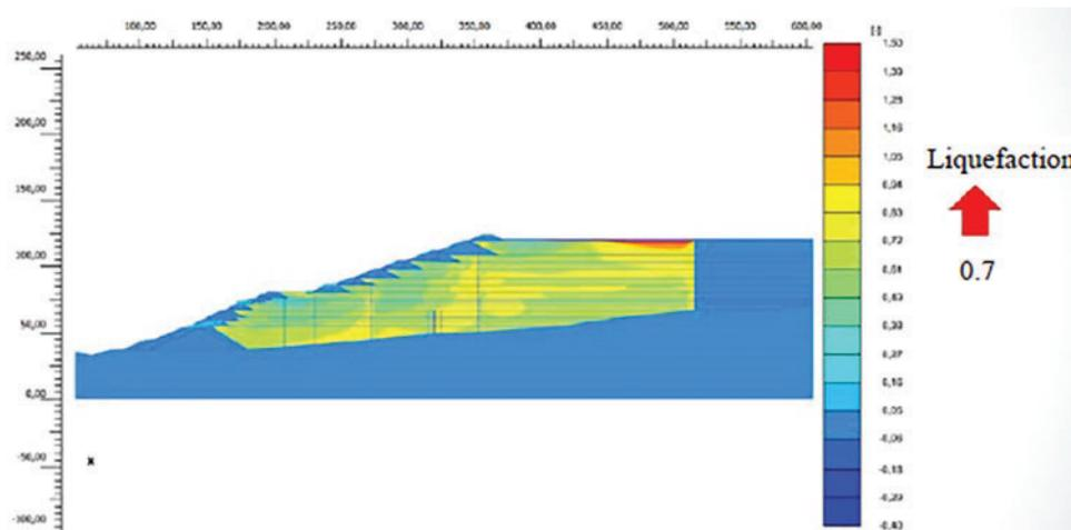
Fig. 15. Liquefaction potential (LP), NorSand model.
