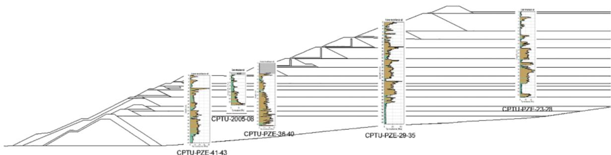
Fig. 11. CPTU's location on the analysed cross-section.
