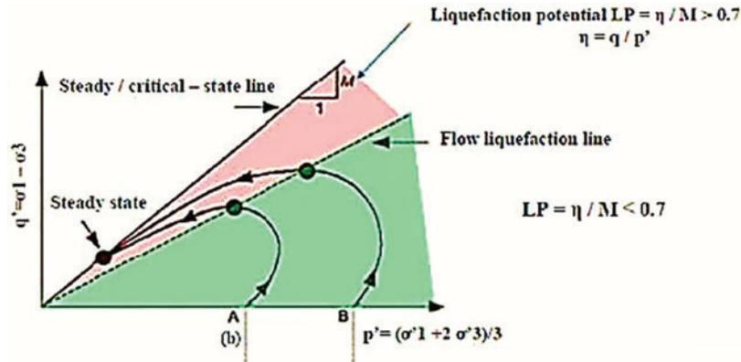
Fig. 9. Definition of liquefaction potential (LP) on the stress path.
