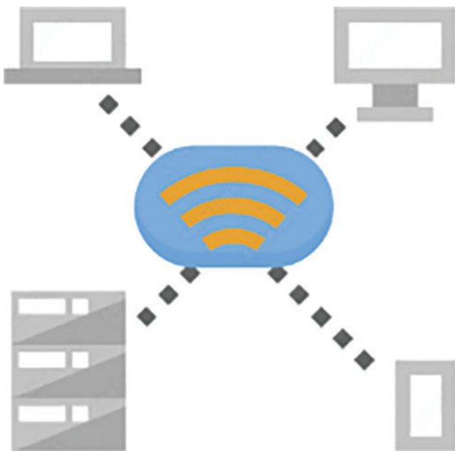
Fig. 7. The Bluetooth creates a network over which not just 2, but several devices can get connected and communicate with one another. A network established over Bluetooth is called Wireless Personal Area Network (WPAN).
