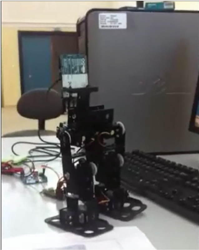
Fig. 1. A simple example of the applied model is BRAT, a 6 degrees of freedom humanoid we have been using in the Lab for students to study bipedal motion.
