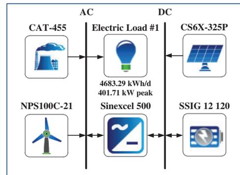
Fig. 6. Schematic diagram of the hybrid power system.
