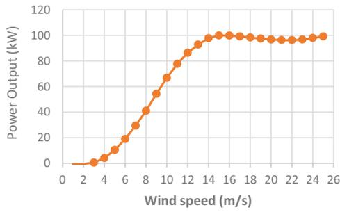
Fig. 5. Power curve graph of the selected wind turbine.
