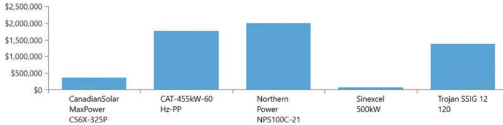
Fig. 7. Detailed description of the net present cost for hybrid PV/WT/DG/BS system.
