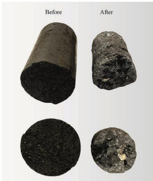
Fig. 9. The change in briquette volume after calcination in a muffle furnace.
