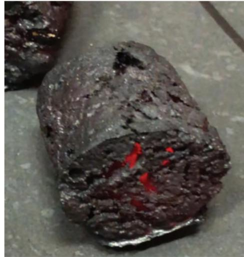
Fig. 6. Photos of the auger pressing briquettes (recipe 1) during laboratory test after 30 min.
