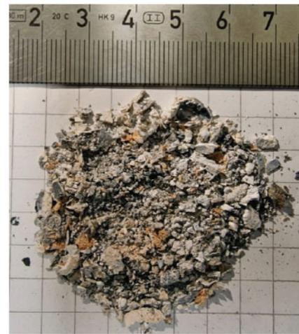
Fig. 14. Zinc oxide concentrate captured by the gas cleaning system.
