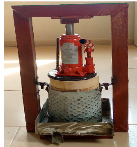
Fig. 4. Honey extractor developed.
