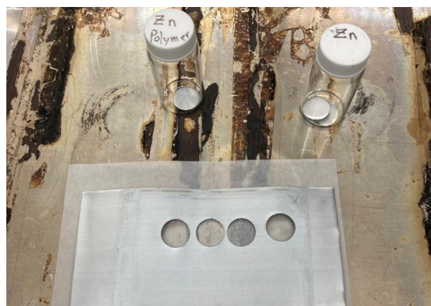
Fig. 4. Anodes cut out by punch and die.
