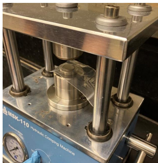
Fig. 6. Crimping machine used to finalize coin cell.
