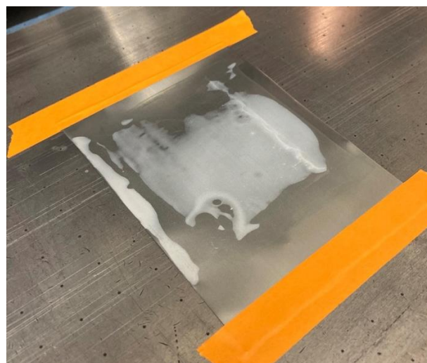
Fig. 3. Polymer coating spread across zinc sheet.
