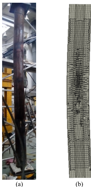
Fig. 2. a) Failure mode of the tested column under steady-state regime; b) Predicted deformed shape.
