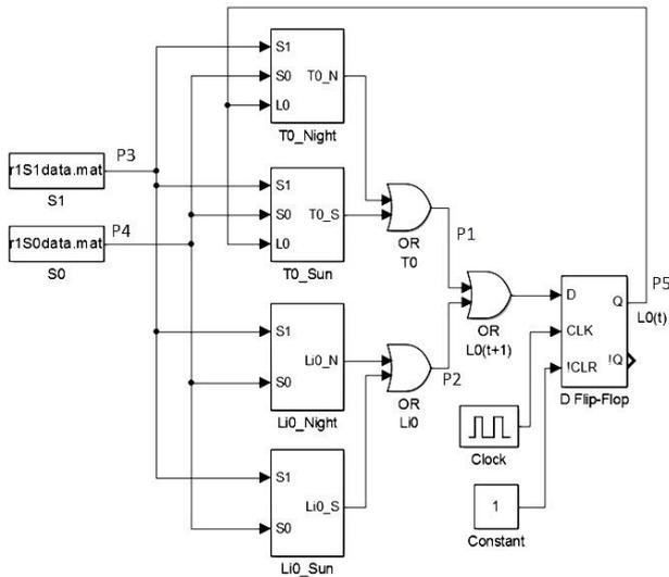
Fig. 7. The whole circuit for the one room design showing points at which probes (P1, P2, P3, P4, P5) are used to take readings.
