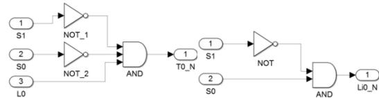
Fig. 5. (L): The circuit for the equation of  $T_{0\_N}$  is shown on the left.
