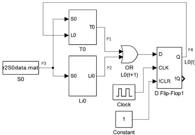
Fig. 11. The whole circuit for room 1 in the two room design showing points at which probes (P1, P2, P3, P4) are used to take readings.
