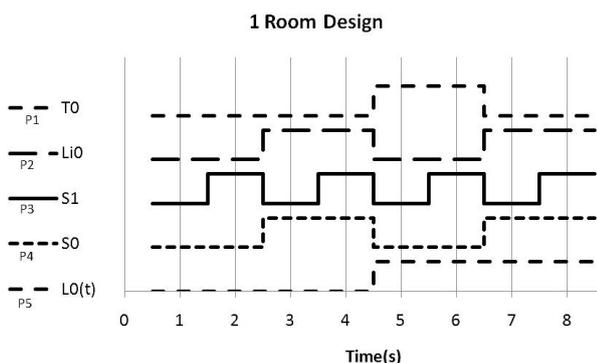
Fig. 8. Input and outputs of the logic circuit shown in Fig. 7 showing the probes at which readings (P1, P2, P3, P4, P5) were taken.
