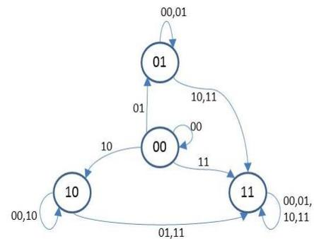
Fig. 4. Mealy state machine for a two room design.
