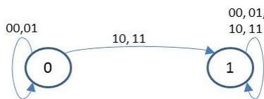
Fig. 2. Mealy state machine for a one room design.
