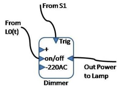
Fig. 9. A Dimmer is used to complete the design in Fig 9.
