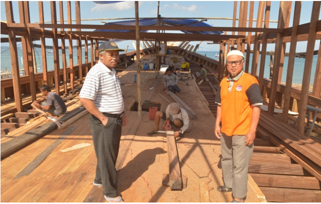
Fig. 2. The stage of working on the floor of the pinisi boat (Researcher is on the floor of the ship).
