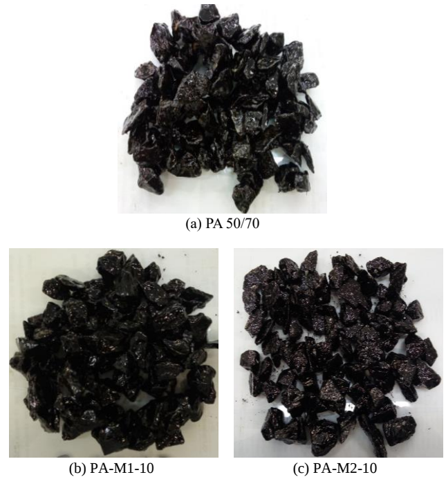
Fig. 5. Photograph of post-adhesive test samples: (a) PA-50/70. (b) PA-M1-10 and (c) PA-M2-10.
