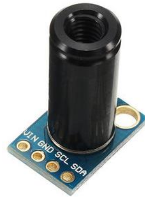
Fig. 5. Infrared temperature sensor MLX90614.
