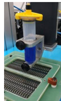
Fig. 4. Adhesive being applied in SMD PCB's.
