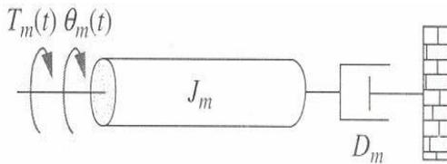
Fig.2 Motor with a mechanical load
