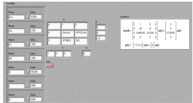
Fig.4 State space model of linear electric motor in LabVIEW.
