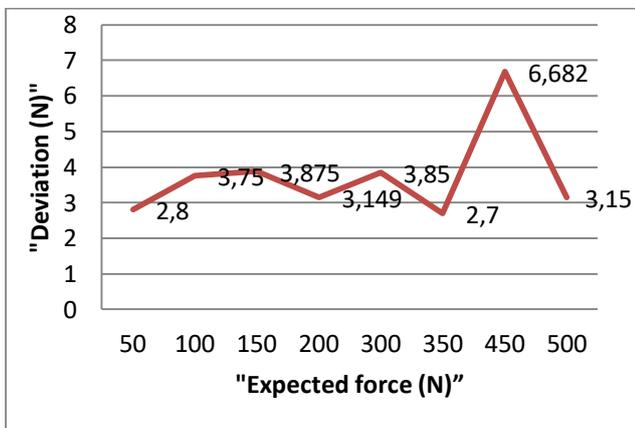
Fig.5 Deviation caused by the load cell at different expected forces
