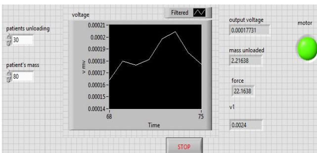
Fig.6 Graph showing the variation in the load cell output, patient's unloading (%) (i.e. required), mass and force unloaded by the load cell
