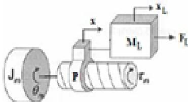
Fig.3 Free body diagram of linear actuator
